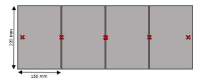
Figure 3. Showing the dimensions and arrangement of one of the sets of four trays along with the positions of the five data loggers, illustrated by the red crosses, used to measure the temperature gradient.
